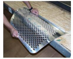
The window guard must be prebent so it fits tight against the contour of the door window frame. The aluminum guard can easily be formed at workbench.
